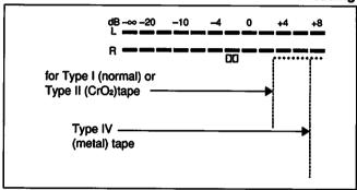
Tips on recording level adjustment
