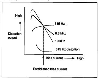
As shown above, characteristics such as output level and distortion differ widely according to the bias (high-frequency) current. In conventional systems, the bias current is susceptible to variations in certain recording signals (see diagram below) which may cause fluctuations in frequency response, distortion, or other unwanted characteristics.
